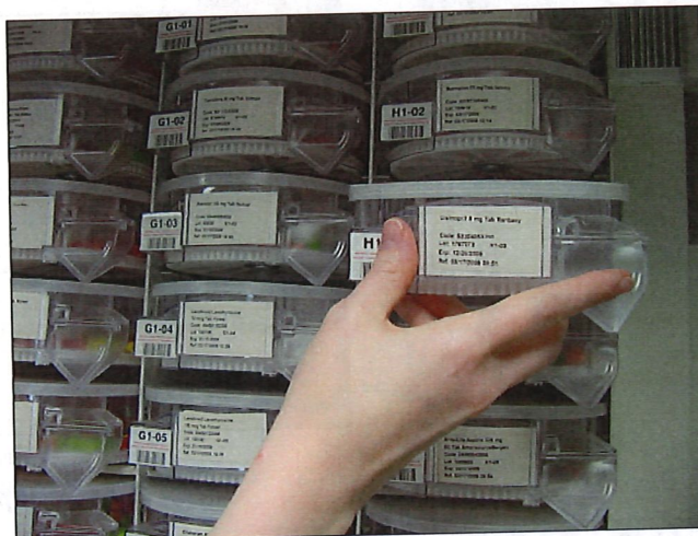
Removing a Cell from the Robotics Cabinet
