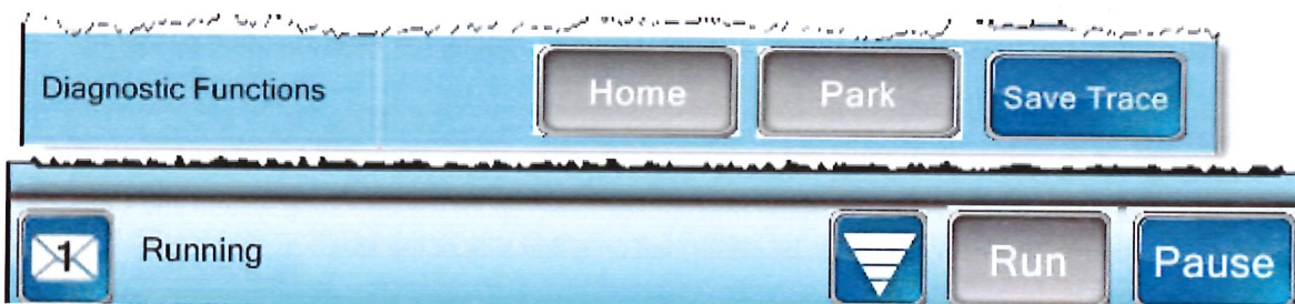
Figure 25: The Home and Park buttons are disabled when the Max is in Run mode.
